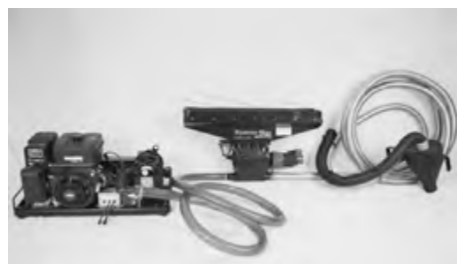
Complete Seed Jet, bulk seed handling system. Safely handles that fragile seed.
